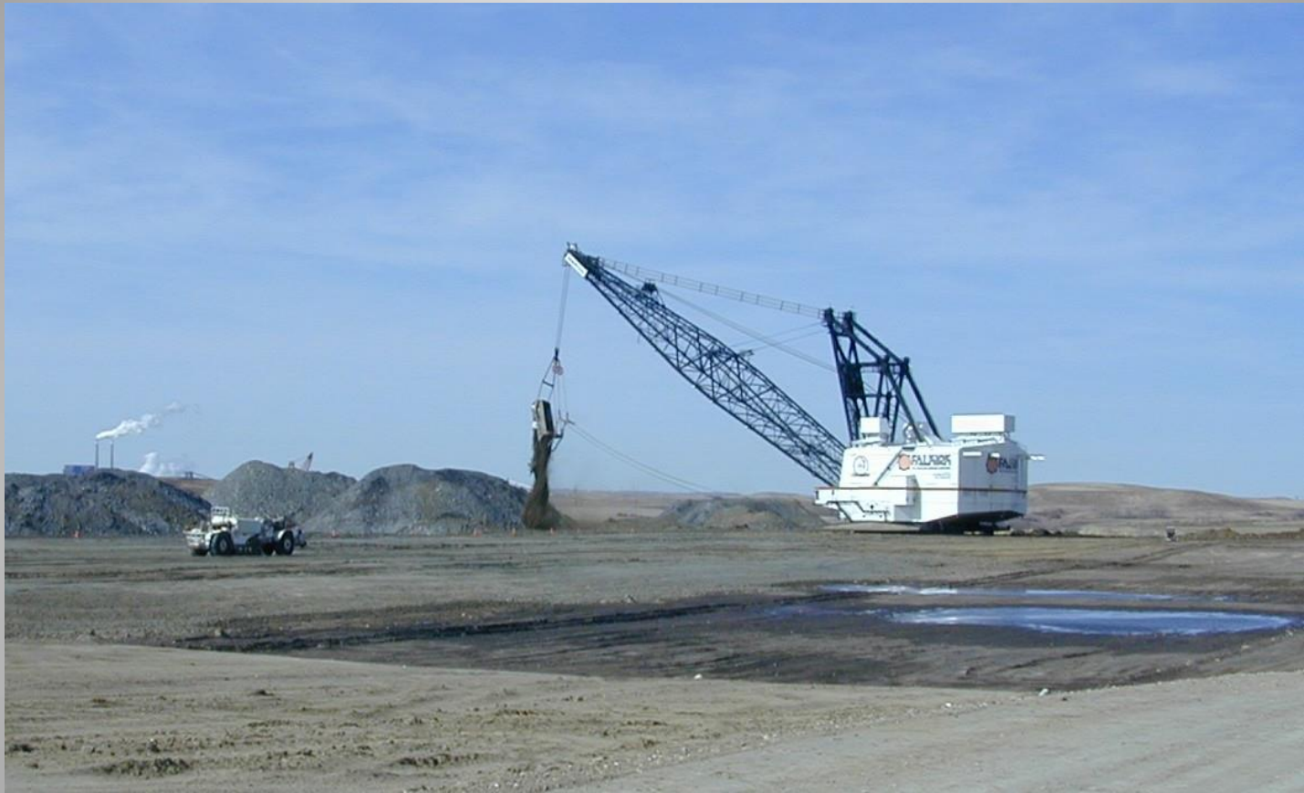
Dragline removing overburden at the Falkirk Mine
