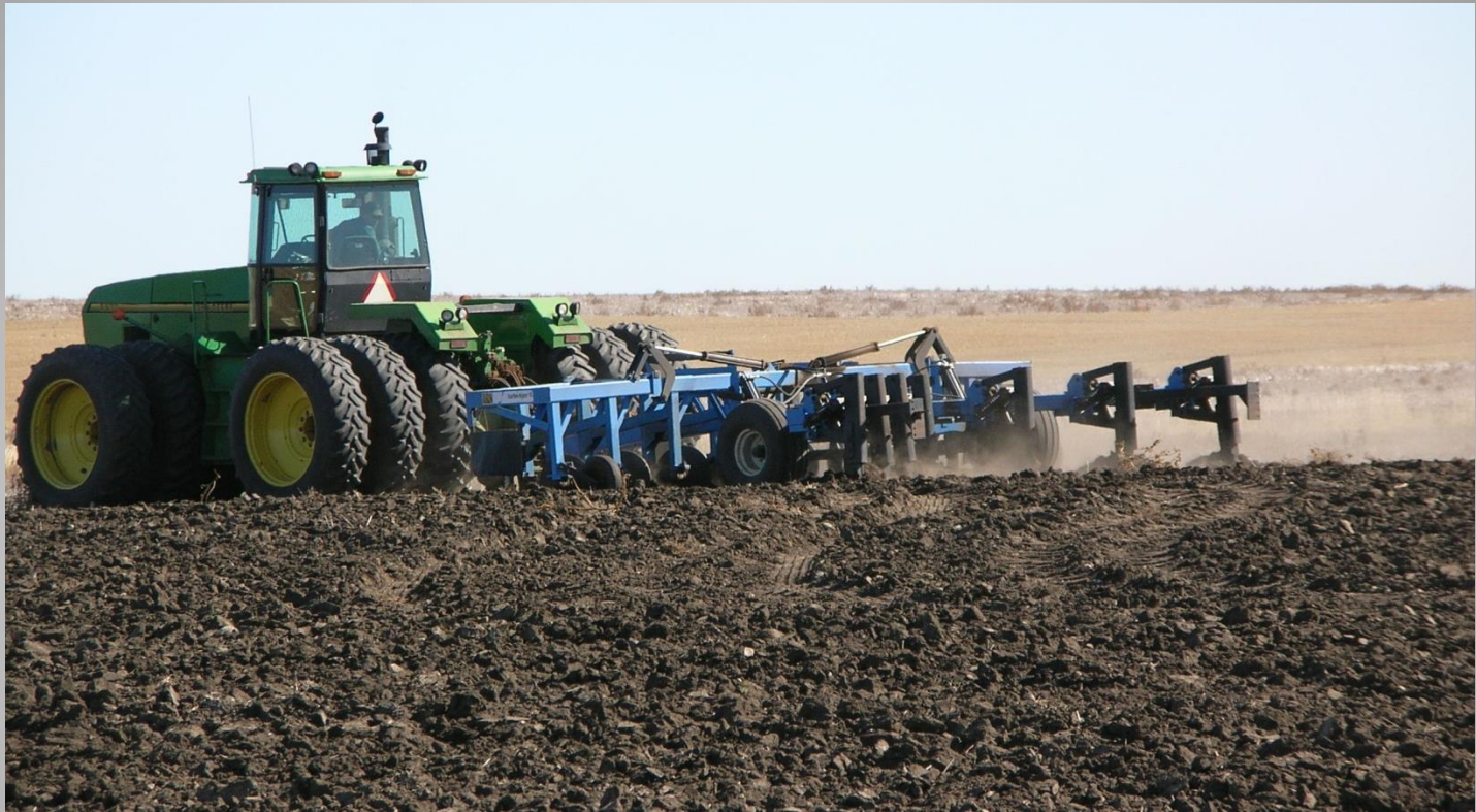
Deep ripping reclaimed cropland to help alleviate subsoil compaction
